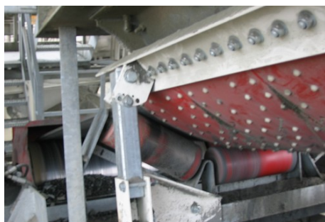
Sand lime - 500 tons per hour 1000 Belt
