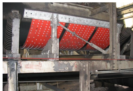
Coal harbour - 3.200 tons per hour 1600 Belt - speed 3,2 m / second
