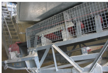
Limestone 300 tons per hour 800 Belt
