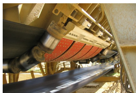
Cement works - 800 tons per hour 1.200 Belt ( 5 hanging straps )
